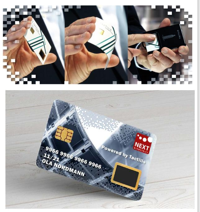
\* Incorporates NEXT NB610 flexible fingerprint sensors compliant with ISO 17839 defining the implementation of biometric system-on-a-card devices
